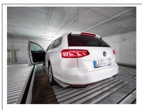
Figure 6: Especially wide parking spaces of 270 cm enable the user to enter and exit the vehicle conveniently.
